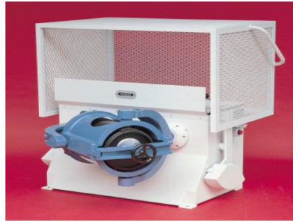
Fig.2 Schatz Shaker Mixer Geometry
